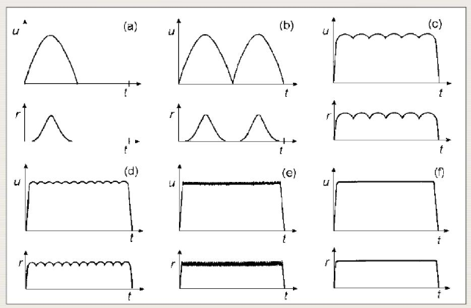
Voltage waveforms u and associated tube output (dose rate) r for (a) 1-pulse (b) 2-pulse (c) 6-pulse (d) 12-pulse (e) high-frequency (f) constant voltage generators
