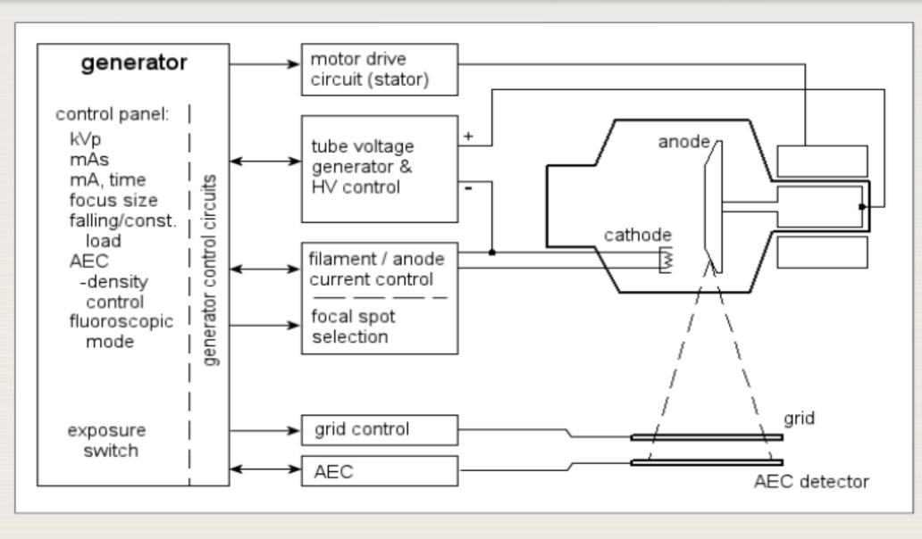
Schematic diagram of a basic X ray generator
