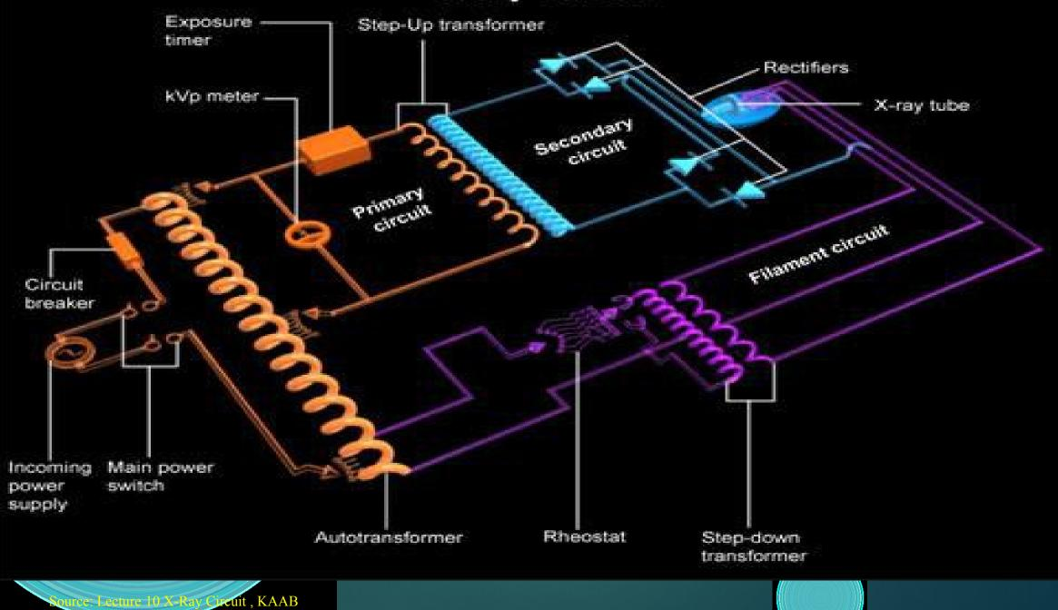
The main circuit and filament circuit are combined to form the complete basic x-ray circuit that is composed of sequence of devices to produce x-rays.
